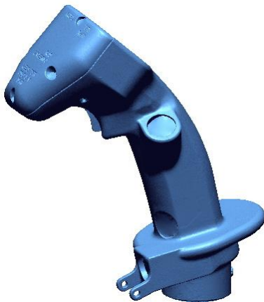
Figure 2 – Laser Scanned Data
